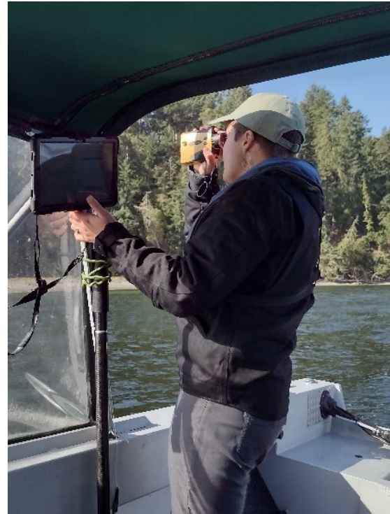
Figure 2.2. Field Staff Conducting Offset Mapping Using a TruPulse 360-Series Laser Rangefinder and Esri FieldMaps Application.
