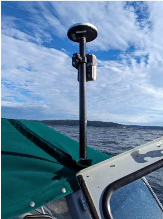
Figure 2.1. EOS Arrow 100 GPS Receiver and Antenna Mounted to the Field Boat.
