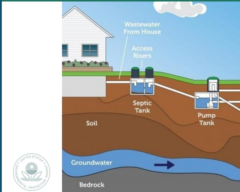
Consisting of a septic tank, pump tank, pump, and drainfield, these types of systems utilize pressure to move wastewater throughout the system. The pump tank is similar to a septic tank in size, and houses a pump and different alarm floats. These systems typically are timer set so the pump doses the drainfield, evenly distributing a set amount of the wastewater to the lines at various times of the day. Pumps, alarms, and panels require electrical hookups and wiring that can also malfunction.
