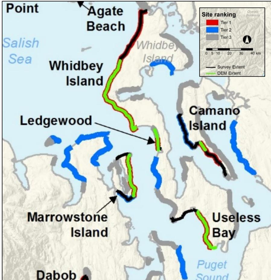
**Figure 1. Spatial Extent of Surveyed Shoreline Versus Processed Data and DEM Development (Weiner et al. 2018).**
