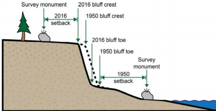
**Figure 2. Bluff Profile Depicting Bluff Features and Survey Monuments Used to Measure Change Rates.**
