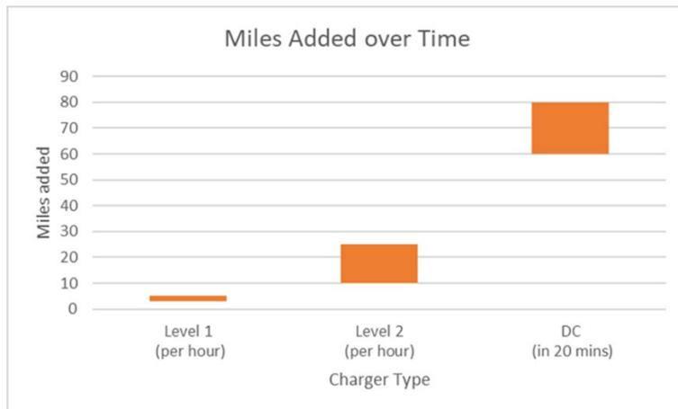
Figure 1: EV Charger Speed Comparison
